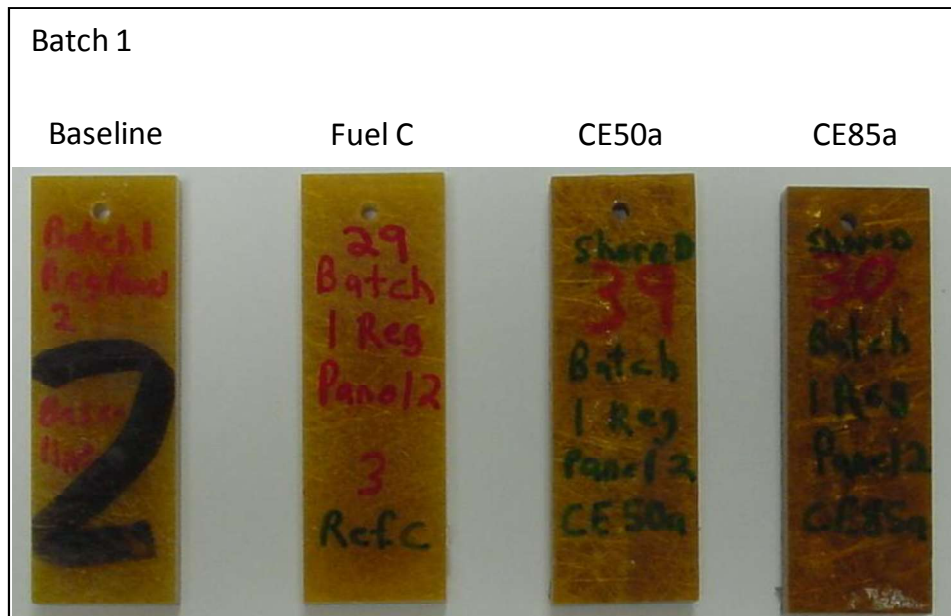
Fig. 12. Photograph showing the Batch 1 specimens before and after exposure to Fuel C, CE50a, and CE85a.
